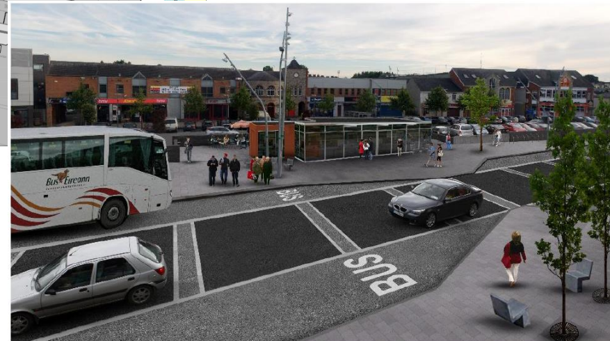
Figure 10: Kennedy Road, incorporating set back bus stops and taxi ranks, increased pedestrian space and potential for a new ticketing/information facility.
